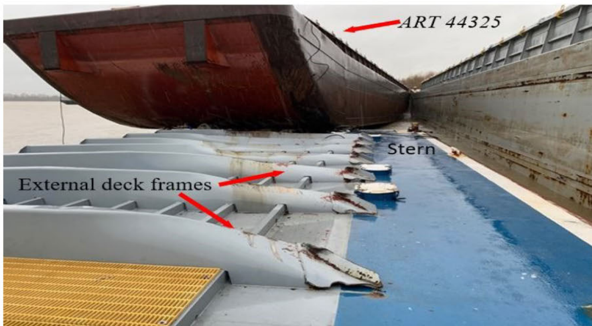
Figure 8. Post-accident damage survey of the RHA 2204 and ART 44325. (McKinney Salvage, LLC, annotated by the NTSB)
